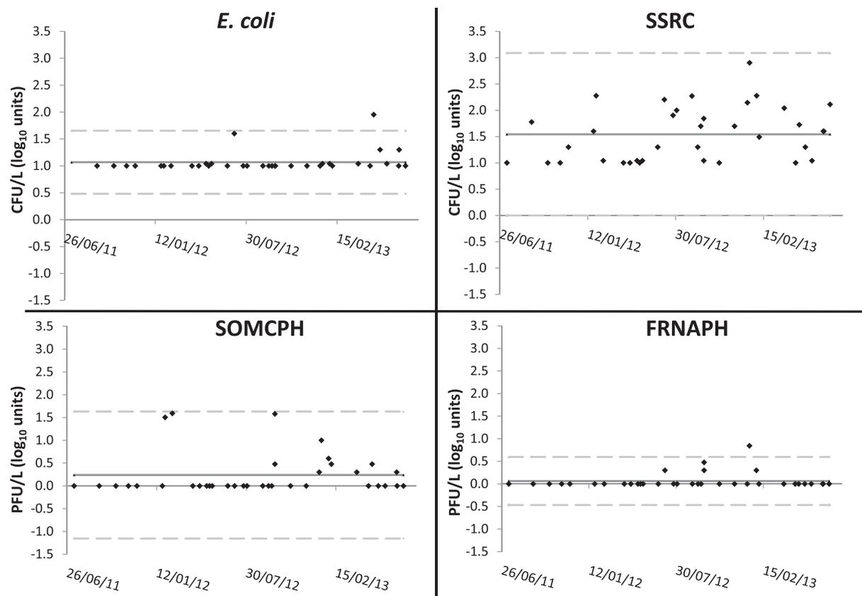
**Fig. 3.** Concentration evolution along time of *E. coli*, SSRC, somatic coliphages SOMCPH and FRNAPH in pre-treated water samples with the dioxichlorination – coagulation/flocculation-settling-sand filtration treatment scheme. Center line (solid) corresponds to the data mean, and the upper and lower lines (dotted) to the mean  $\pm 3\sigma$  standard error, respectively.
