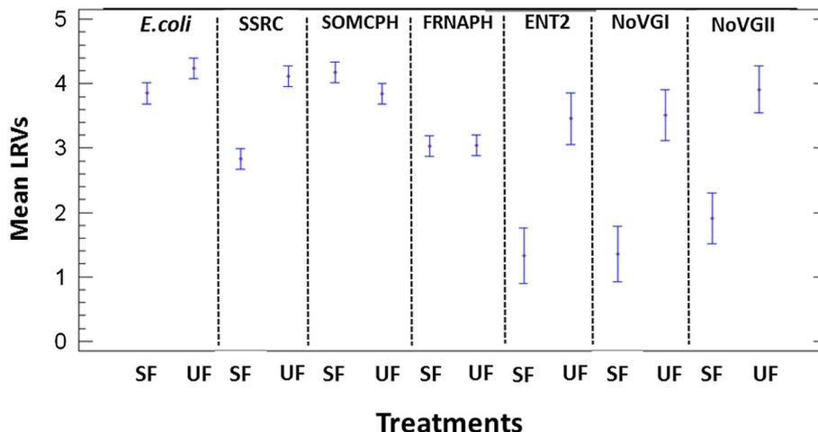
Fig. 5. Mean LRVs of *E. coli*, spores of sulfite reducing clostridia (SSRC), somatic coliphages (SOMCPH), F-specific RNA coliphages (FRNAPH) ENT2, NoV GI and NoV GII, for direct UF (UF) and conventional pre-treatment, (SF); schemes obtained during the two year period considered.
