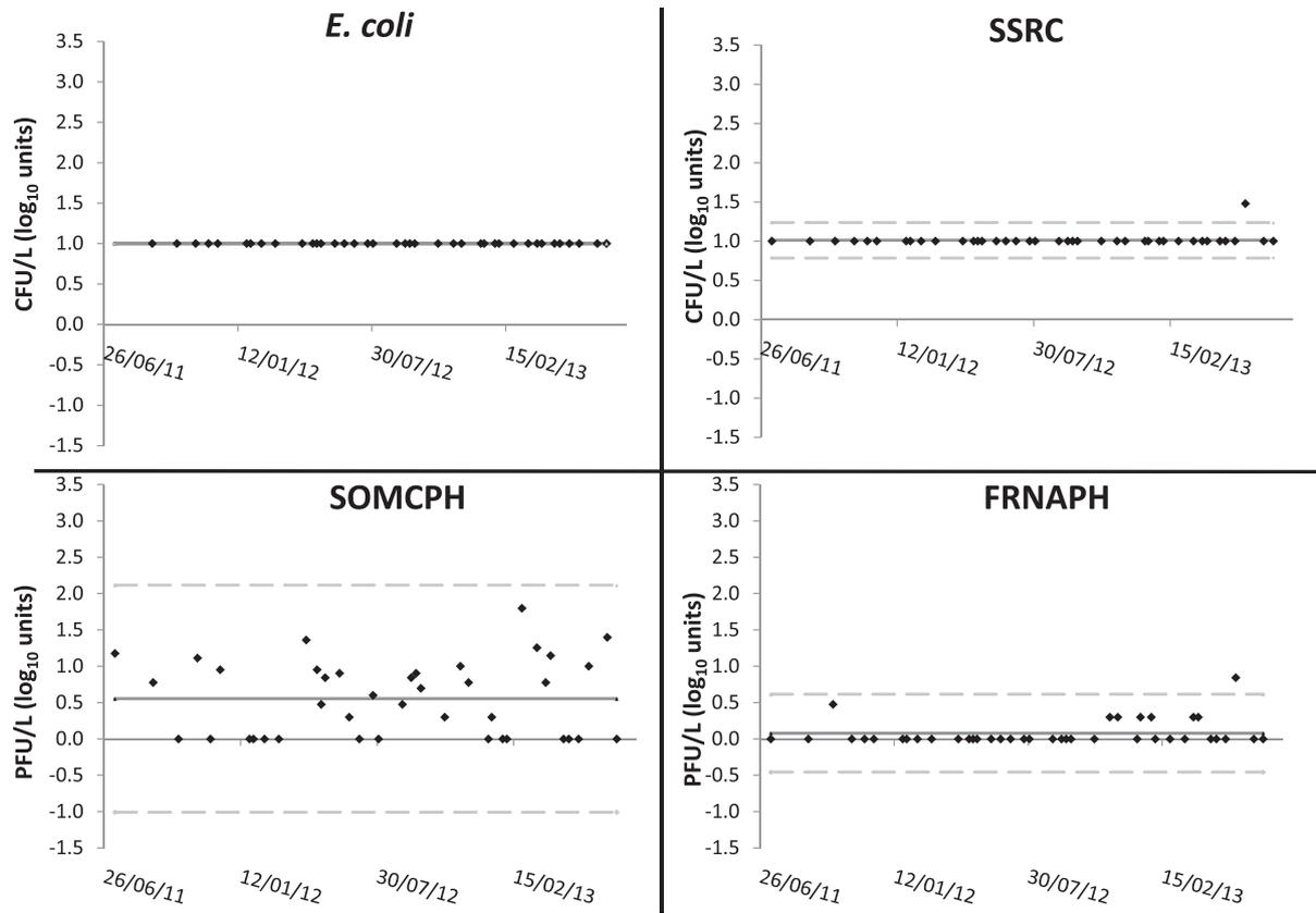
Fig. 4. Concentration evolution along time of *E. coli*, SSRC, SOMCPH and FRNAPH in the ultrafiltered water (direct UF treatment scheme). Center line (solid) corresponds to the data mean, and the upper and lower lines (dotted) to the mean  $\pm 3\sigma$  standard error, respectively.
