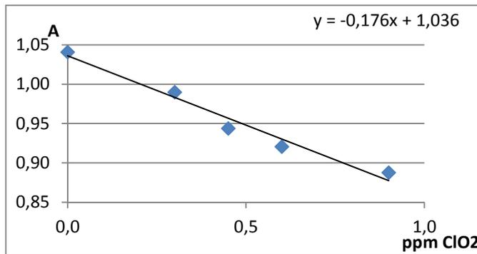
Figure 1. A typical calibration curve for chlorine dioxide analysis by LGB method.
